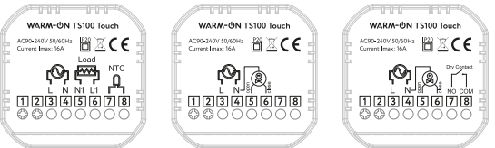
WE electrical heating WW water heating WW-LD boiler heating and water heating
